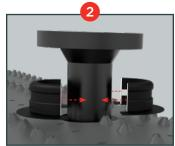
**STEP 2A** Install left and right sides of the Integrity Pipe Seal around the pipe protrusion.
