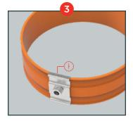
**STEP 3** Align the joiner to the center of the 1/8" gap at the 6 o'clock position.
